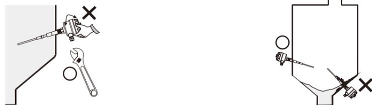
X: Do NOT use enclosure to thread probe into its process connection
